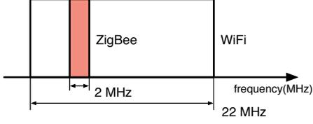
Fig. 5. Channel bandwidth of ZigBee and WiFi
