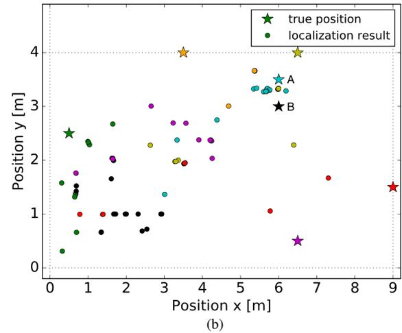
Fig. 12. Localization results of ZigLoc (a) without and (b) with differential fingerprinting. Stars are true target locations. Circles indicate localization results and the color represents the corresponding true location.
