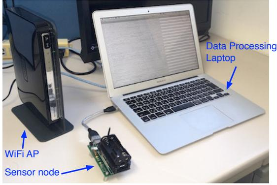
Fig. 8. Sensor node, WiFi AP, and data processing laptop used in implementation
