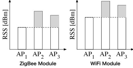
Fig. 6. RSS offset between ZigBee and WiFi modules
