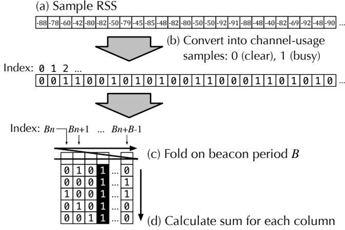
Fig. 2. Overview of AP signal detection. (a) A sensor node samples RSS and (b) converts the RSS samples into channel-usage samples. (c) The sensor node folds the channel-usage samples on beacon period, and (d) calculates the sum for each column to get channel-usage sums. Periodic beacon signals appear in a specific column, resulting in a large channel-usage sum.
