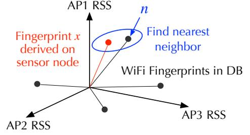
Fig. 3. Basics of ZigLoc fingerprinting localization
