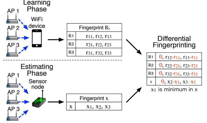
Fig. 7. Overview of differential fingerprinting
